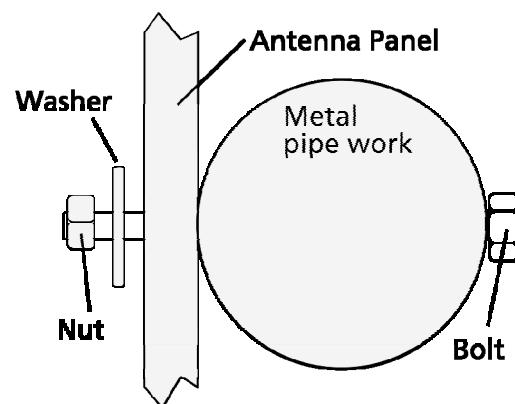
4. Using the **defined mounting holes**, mount the Antenna Panel on the **outside** of the animal handler so that the middle of the Antenna Panel matches the average height.
