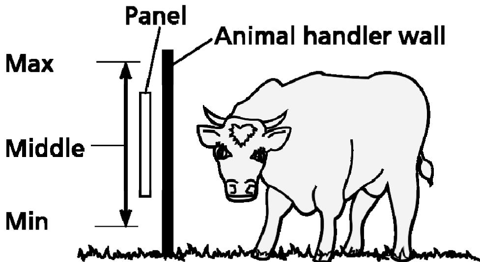
2. Determine the average height of the Electronic ID and mark this on the **outside** of the animal handler.
