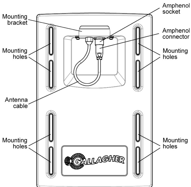
**Note:** You may want to temporarily attach the Antenna Panel and test the read range prior to permanently attaching the Antenna Panel.
