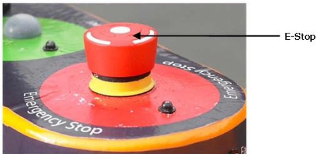
Figure 18. E-Stop button position.
