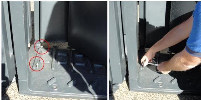
Figure 9. Attaching to Sheep Auto Drafter.
