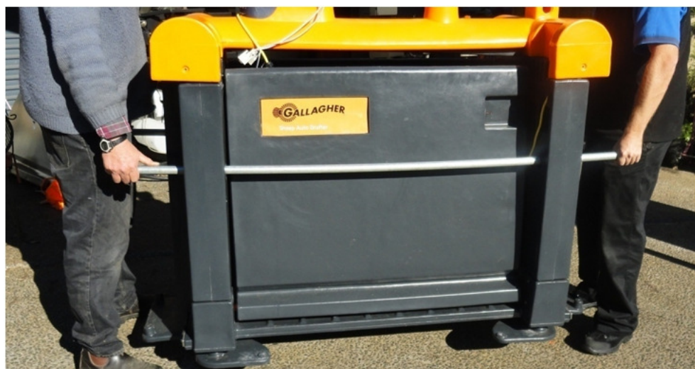
Figure 6. Lifting using the transport poles.
