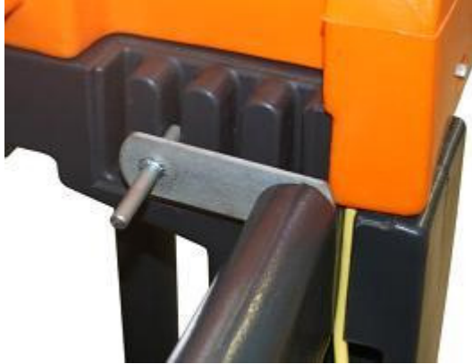
Figure 17. Slots and locking lever to allow Sheep Auto Drafter width adjustment.
