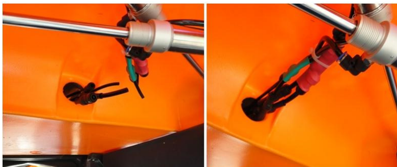
Figure 10. Attaching air lines.
