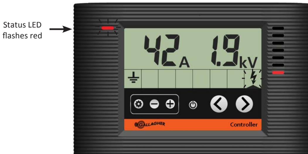
Controller showing the energizer in current alarm
