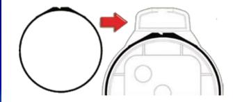
To insure waterproofing, keep both rubber seals positioned correctly on top and bottom of the unit.
