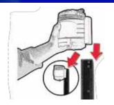
The preferred method to mount your FoxlightS is on the back of a star post placed in position to maximize field coverage.
