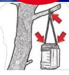
With a strong tie to a beam or tree branch. (Note the tree trunk will obscure the light in its direction)
