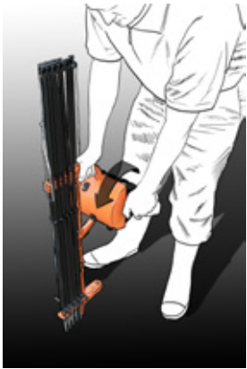
STEP 1 Loosen lock nut (anti-clockwise).
