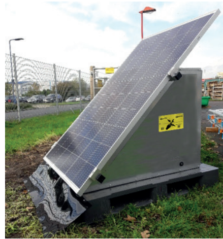
Figure 3.1: PVC strip prevents shadows on the solar panel caused by grass growth
